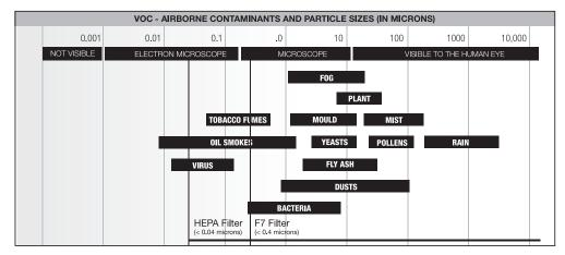
All SmartVent systems feature high grade F7 filters\* that capture up to 90% of 0.4 microns particles such as fine pollens, dusts and allergen from the air making the air cleaner to breathe. High quality HEPA filters are also available for asthma and allergy sufferers.
